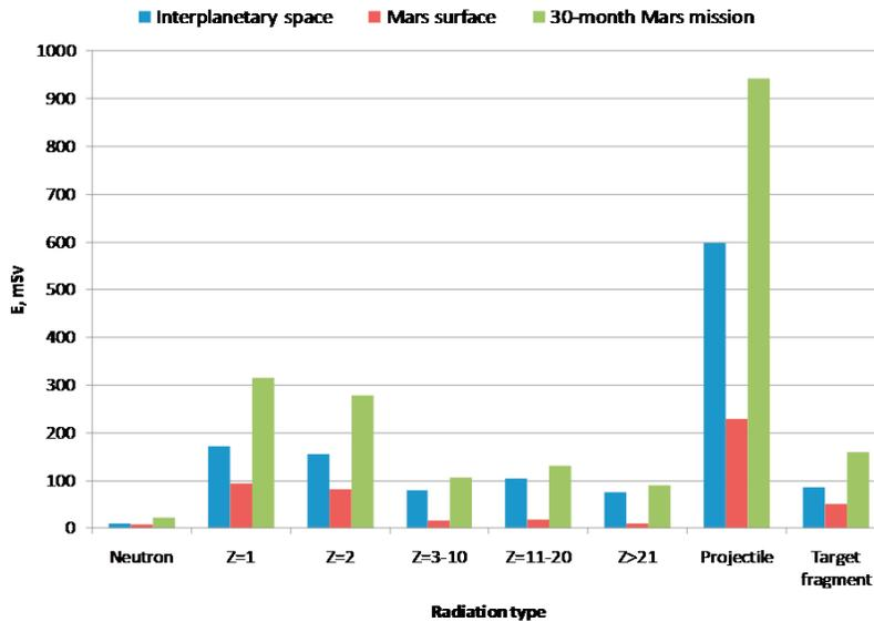
Figure 4. Effective doses for GCR charge groups, the overall projectile-like effective dose (primaries and projectile fragments), and of target fragments inside a spherical spacecraft of 5 g/cm<sup>2</sup> aluminum shield thickness: annual exposure in interplanetary space and on Mars surface and that for 30 month Mars mission.
