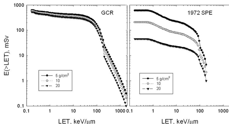
**Figure 1.** Integral LET distribution of (left) effective dose for annual GCR at solar minimum and (right) the 1972 SPE behind several thicknesses of aluminum shielding.
