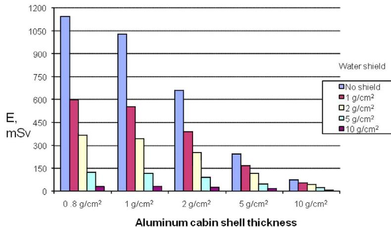
**Figure 2.** Effective dose analysis of lunar rover concept with water shield augmentation for optimization of shield mass and effective dose reduction.
