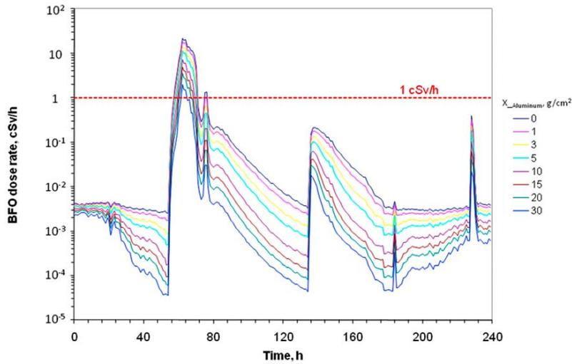
Figure 3. Calculations for the 1972 SPE of the BFO dose equivalent rate versus time for increasing amounts of aluminum shielding. The calculations show that intermediate dose equivalents rates are reached if only thin shields are available.
